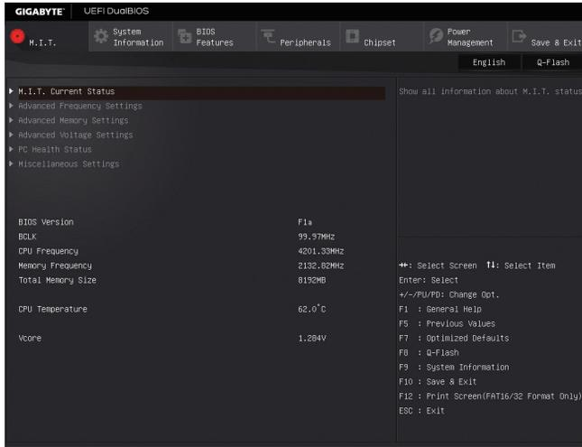
This section provides information on the BIOS version, CPU base clock, CPU frequency, memory frequency, total memory size, CPU temperature and CPU voltage, etc.
