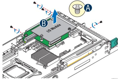
**Figure 46. Removing the IOM Riser and Carrier Assembly**
