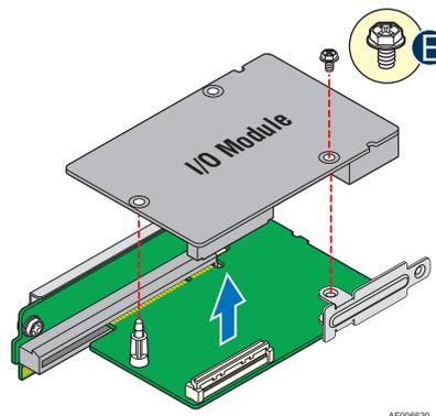
**Figure 48. Removing the IO Module from the IOM Riser and Carrier Assembly**
