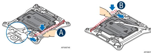
**Figure 13. Installing the Processor – Open the Socket Lever**
