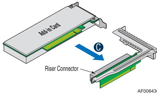
**Figure 38. Installing the PCIe Add-in Card**
