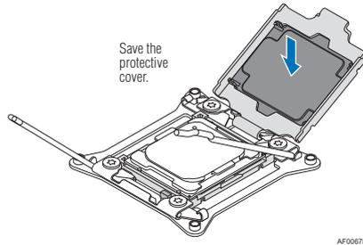
**Figure 16. Installing the Processor – Remove the Cover**
