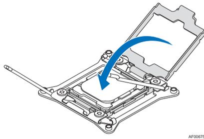
**Figure 17. Installing the Processor – Close the Load Plate**
