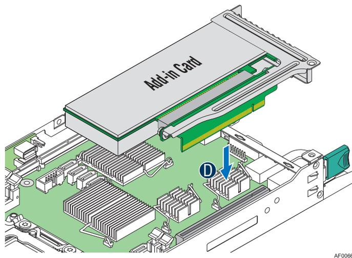
**Figure 39. Installing the PCIe Riser Assembly – Step 1**
