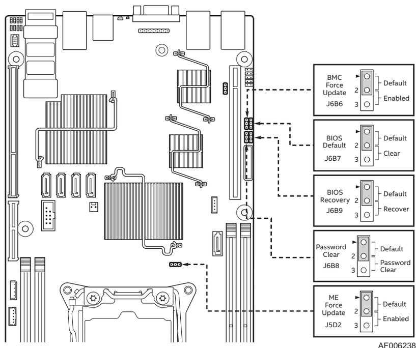
**Figure 8. Configuration and Recovery Jumpers**
