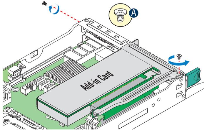
**Figure 27. Removing the PCIe Riser Assembly – Step 1**
