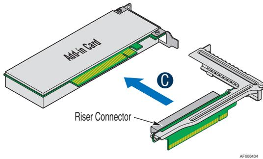
**Figure 35. Removing the PCIe Add-in Card**
