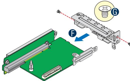
**Figure 49. Installing the Bracket to the IOM Riser and Carrier Assembly**
