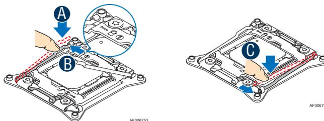
**Figure 18. Installing the Processor – Latch the Locking Lever**
