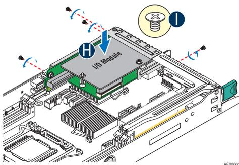
**Figure 45. Installing the IOM Riser and Carrier Assembly**
