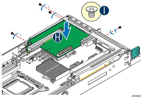
**Figure 50. Installing the IOM Riser and Carrier Assembly**
