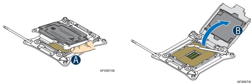
**Figure 14. Installing the Processor – Open the Load Plate**
