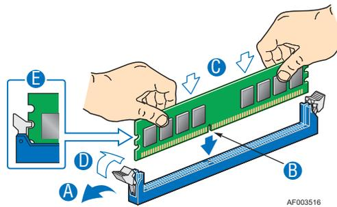
Figure 20. Installing the Memory
