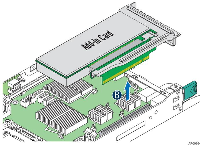
**Figure 28. Removing the PCIe Riser Assembly – Step 2**
