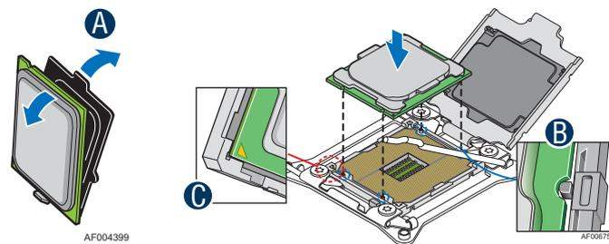
**Figure 15. Installing the Processor – Install the Processor**
