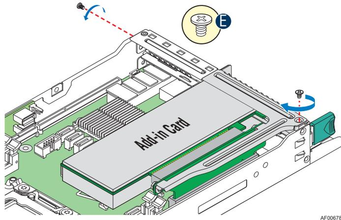
**Figure 40. Installing the PCIe Riser Assembly – Step 2**
