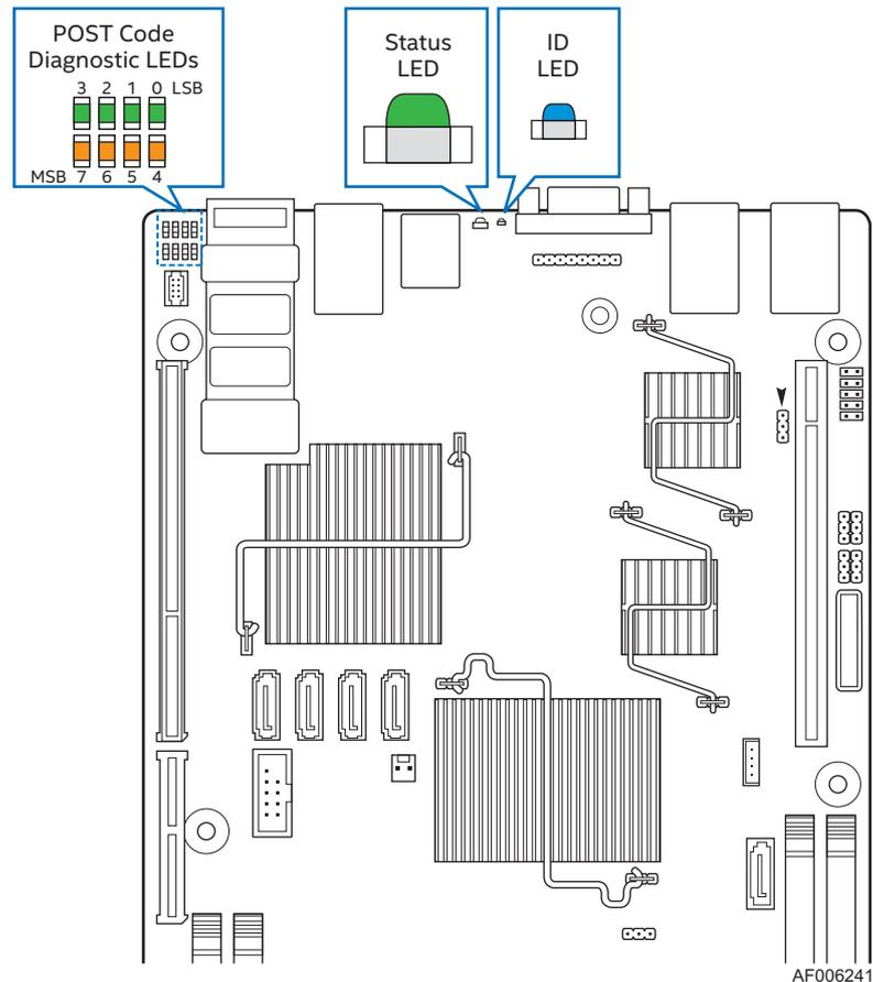
**Figure 7. Intel® Light-Guided Diagnostic LEDs – Server Board**
