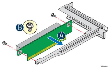
**Figure 37. Installing the PCIe Riser to the Riser Assembly Bracket**
